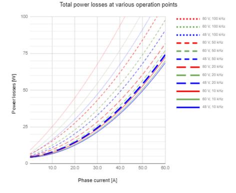
Following figure show the theoretical **power losses** at different operating points.
