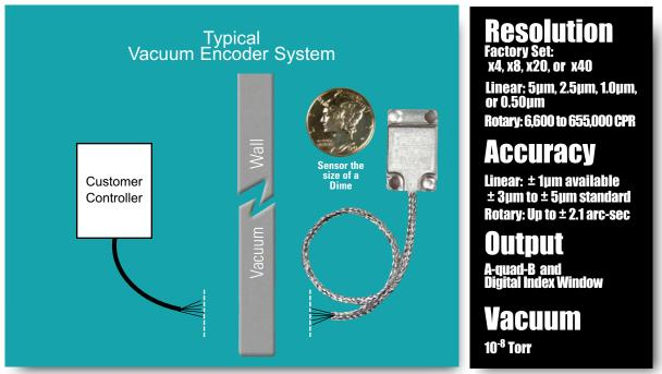
The New Mercury 1500V Digital Output Vacuum Encoder is a cost effective solution with high immunity to EMI noise and all digital outputs straight from the sensor.
